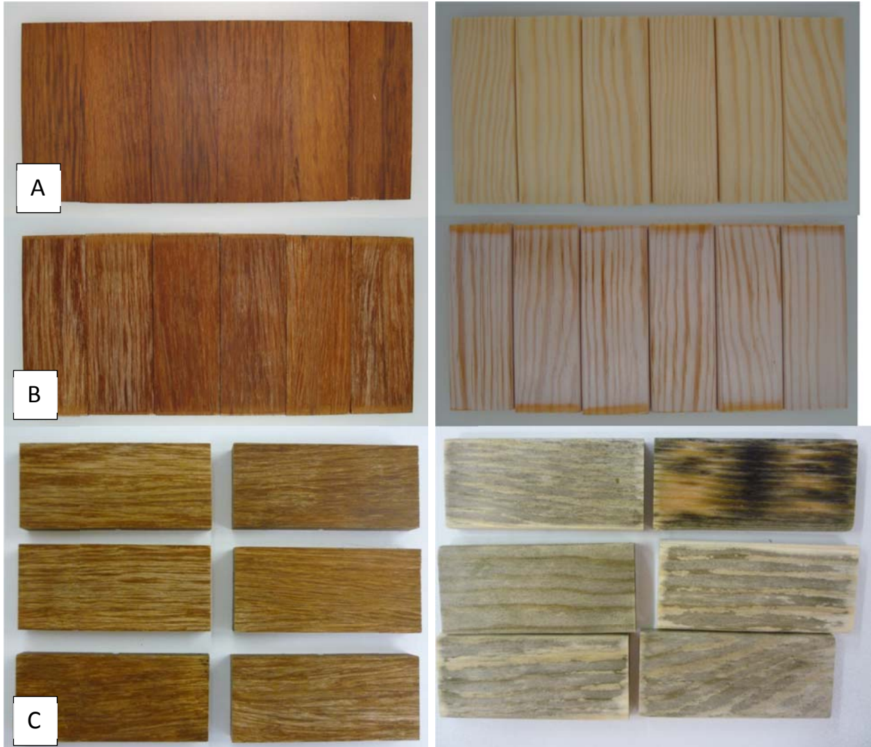
Figure 1: Surface of test specimens (left side) and reference specimens of pine sapwood (right side), before (A) and after (B) 4 weeks of QUV weathering and after 6 weeks of attack by blue-stain fungi (C)
