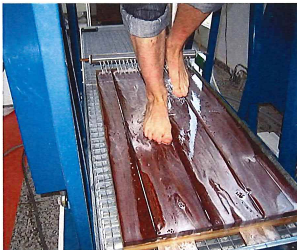
Fig. 1: Wet deck boards during the test on the ramp test
